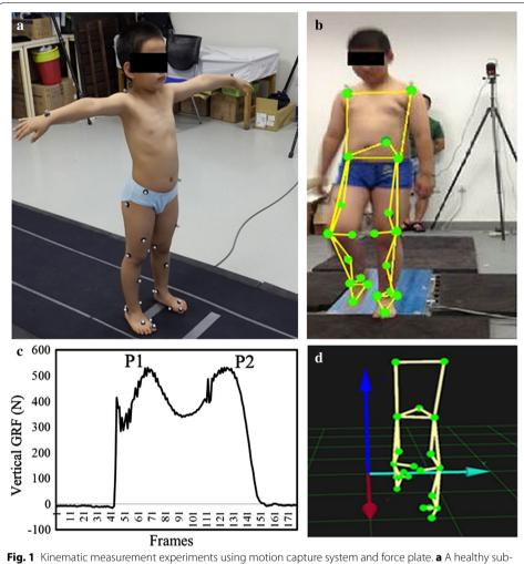
**Fig. 1** Kinematic measurement experiments using motion capture system and force plate. **a** A healthy subject under static stance situation. **b** An obese knee valgus subject under walking condition. **c** and **d** Shows the data collection progress. P1 and P2 in *figure* **c** are the first peak and second peak of vertical GRF
