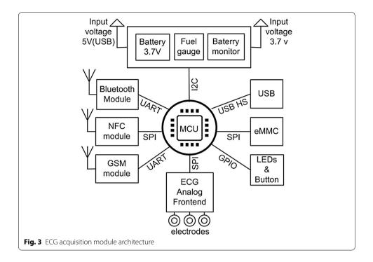
transmission module, a GSM transmission module, one button and indicating Light-emitting diodes (LEDs), a near field communication (NFC) module, and, finally, a USB I/O port for charging, testing, and wired file transmission. Universal asynchronous receiver/transmitter (UART) communication is implemented to to enable the communication between the GSM and the MCU modules.
