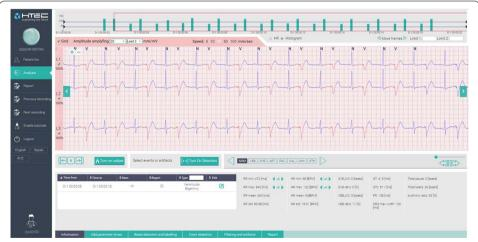
**Fig. 6** Screen-shot of the web analysis platform. Automatic analysis results are seen in the *bottom part*, while the signal is shown with *colors* annotating the beats classification. Physicians have an access to their patients recordings so they can confirm the automatic analysis results and follow their status
