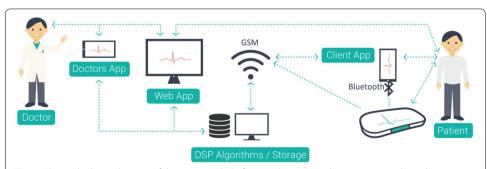
**Fig. 1** Shows the basic diagram of the presented platform and its principal components, where the proposed device is wirelessly transmitting the recordings to a handheld mobile phone which transmits the signals to a cloud server. Signals could be directly transmitted to the cloud server using GSM connection
