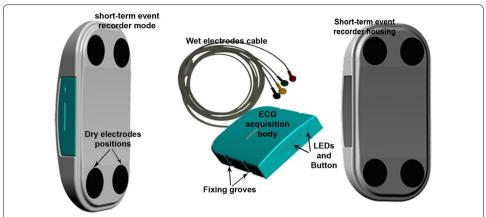
**Fig. 2** Shows the principal components and mechanical design of proposed ECG device, where short-term post-event recorder is enabled b inserting the ECG acquisition body in the short-term post-event recorder housing. Holter or long-term recording mode is enabled by connecting the cable of wet adhesive electrodes to the ECG acquisition body
