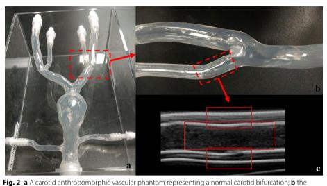
rig. 2 a A carotio anthropomorphic vascular phantom representing a normal carotio birurcation; **b** tr enlarged image of carotid bifurcation; **c** the ultrasound contrast image of external carotid artery
