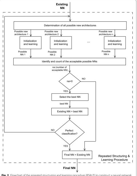
**Fig. 2** Flowchart of the repeated structuring and learning procedure (RS&LP) to construct a neural network (NN) for serial ECGs analysis
