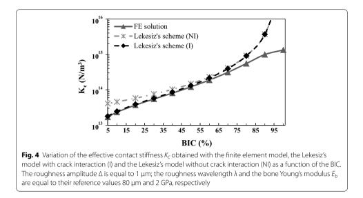
function of the BIC. In this case, the numerical stiffness has been calculated assuming  $\Delta = 1 \ \mu m$  to compare the FE solution with the analytical solutions by Lekesiz, which are valid in the case of crack-like non-contact zones (see "Lekesiz's models" section). All other parameters in the FE model are taken equal to their reference values. The effective contact stiffness is shown to increase as a function of the BIC for all three models.
