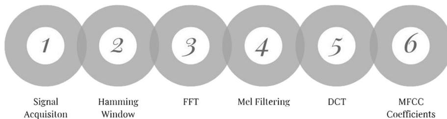
**Fig. 8** MFCC Calculation pipeline [18]
