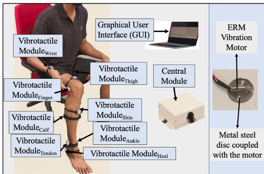
**Fig. 7** Experimental Setup with anatomical locations marked for Vibrotactile modules
