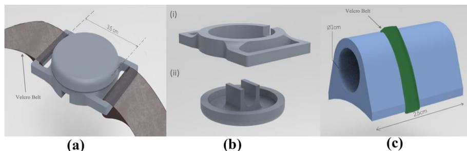
**Fig. 6** **a** The Vibrotactile Module casing (circular) **b** Detailed view of the casing having (i) Base Holder and (ii) Cover, **c** The Vibrotactile Module casing (cylindrical)
