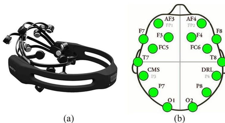
**Fig. 6** Emotive epoch + device. **a** Headband. **b** Electrode locations
